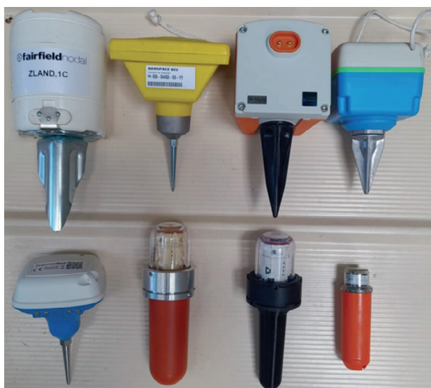
A selection of nodes used for seismic surveys (source: Tim Dean)
